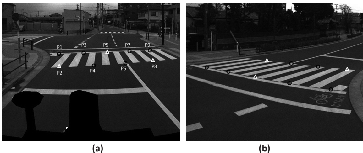
Figure 9. Images taken at the corner by the Ladybug3 system with nine GCPs, in which three white triangles represent control points and six black circles represent check points: (a) part image from lens No.0 (front view); and (b) from lens No.3 (back-side view).
